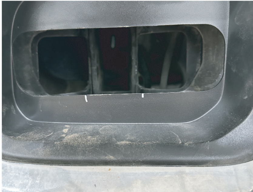
STEP 2A: Mark Bumper for trimming so frame bracket has clearance
