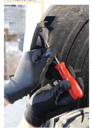
STEP 2: REMOVE 2 BODY PINS EACH SIDE BOTTOM OF BUMPER
