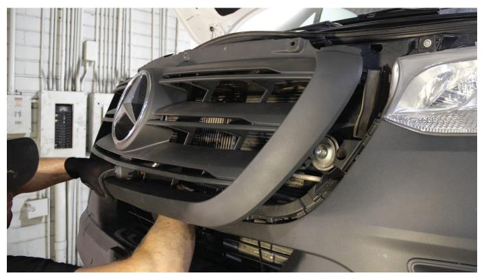
STEP 8: REMOVE THE 2 BOLTS SECURING THE BOTTOM OF THE BUMPER
