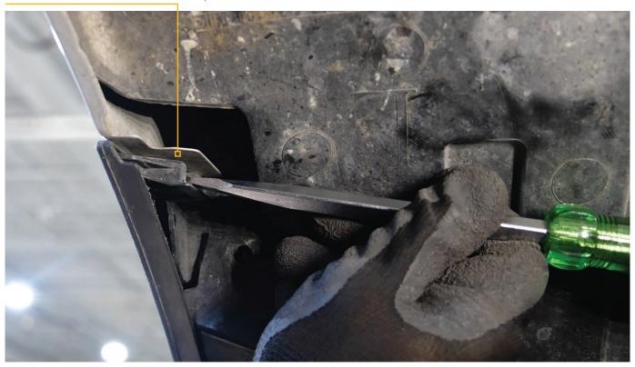
STEP 4: PULL BUMPER SKIN AWAY FROM FENDER, ENOUGH TO REACH IN AND DISCONNECT THE DRIVING LIGHT CONNECTION AND PARKING ASSIST CONNECTION IF EQUIPPED.
