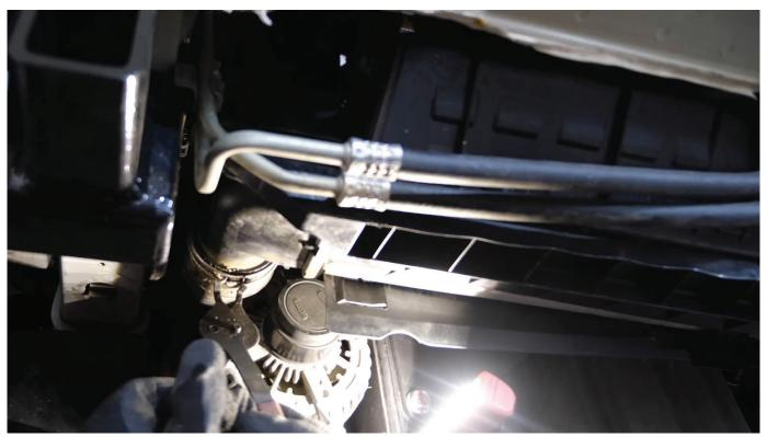
STEP 16: REMOVE THREE BOLTS SECURING FACTORY BRACKET
