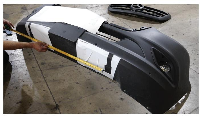
STEP 25: DRILL A 1/2" HOLE ON EACH OF THE CIRCLE LOCATIONS ON THE TEMPLATE.
