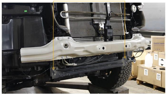
STEP 12: THERE IS A BOLT ON THE DEF TANK THAT NEEDS REMOVE TO PIVOT THE TANK OUT OF THE WAY TO ACCESS THE BRACKET. PASSENGER SIDE ONLY
