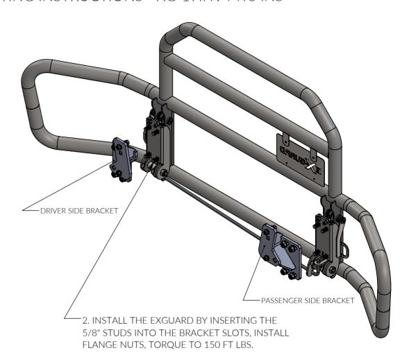
1. REMOVE THE DRIVERS SIDE; TWO BOLTS THAT HOLD THE BUMPER ONTO THE FRAME INSTALL DRIVERS SIDE BRACKET USING BOLTS SUPPLIED, TORQUE TO 110 FT/LBS. REPEAT FOR OTHER SIDE. NOTE DO NOT REMOVE ALL FOUR AT SAME TIME AS THE BUMPER WILL COME COMPLETELY OFF.
