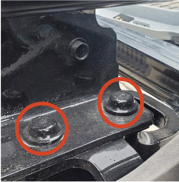
Visual reference of rivets: grind heads off or cut bottoms off to remove
