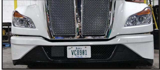
8. Install the Ex-Guard brackets through the bumper and into the receiver. The tow hook should be towards the center of the truck, and the bracket sloping down as shown.
