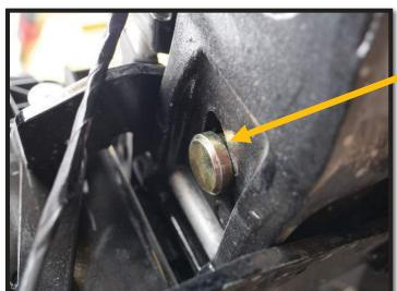
9. Insert the retaining clevis pin through the frame and bracket as shown. And insert the locking ring cotter pin to secure it.
