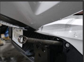
11. Put bumper back in place and torque these 2 bolts per side to factory spec, then proceed to mount the Ex-Guard!
