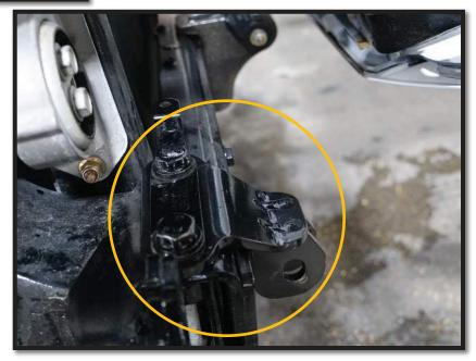
5. Repeat on the Drivers side. Use a pry bar to flex the bracket supporting the wire harness, then locate these 2 bolts and remove them.
