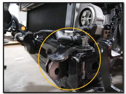
7. Put the bumper back in place, but do not put the 4 bolts in at this time. As you will have to move it, to complete the
