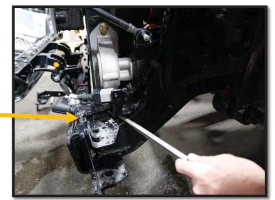
6. Install the top support brace, by placing on the frame and reinserting the bolts and wire support bracket, torque to 225 ft/lbs
