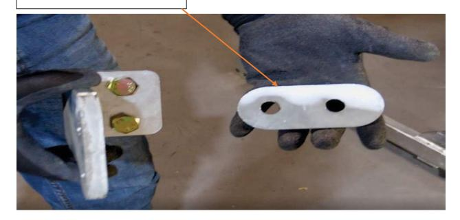
STEP 6: INSERT THE PLATE USING THE HHCS ½"-4.00 LONG BOLT SHOWN BELOW INSIDE THE TRUCK
