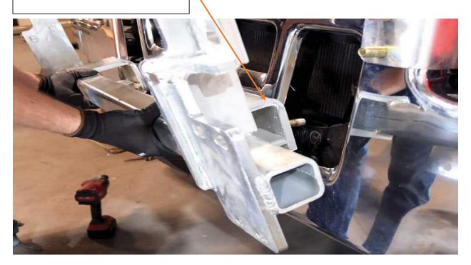
STEP 12: USING THE PROVIDED HARDWARE, TIGHTEN UP THE BOTTOM NUT AS SHOWN
