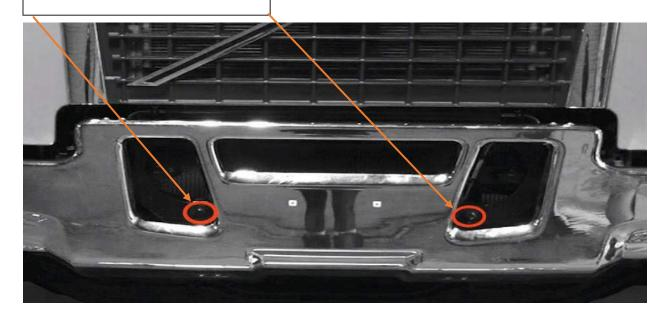
STEP 3: LOOK INSIDE THE TRUCK AND REMOVE THE BOTLS SHOWN BELOW
