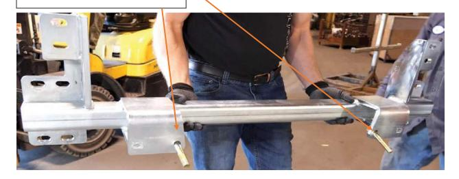
**STEP 11**: INSERT THE BRACKET USING THE PROVIDED BOLT ONTO THE TRUCK
