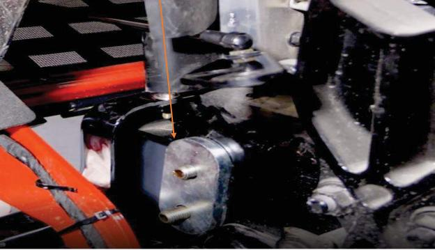
STEP 7: INSERT THE MOUNTING BRACKET XG-17VHD-BR01L & R, ONTO THE PLATE AS SHOWN
