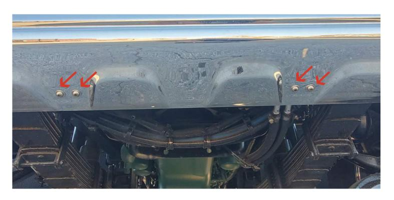
Lift the truck hood and remove the bolt on the left and right side of the bumper. See below:
