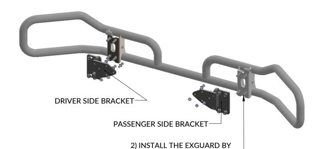
INSERTING 5/8" STUDS INTO BRACKET SLOTS, INSTALL FLANGE NUTS AND TORQUE
