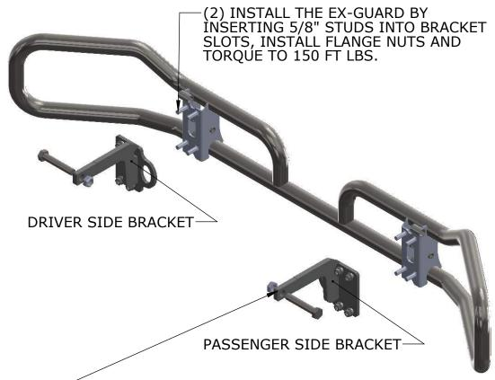
(1) INSERT BRACKETS INTO TOW HOOK RECEIVERS IN TRUCK. THEN INSERT BOLT AND NUT TO SECURE INTO PLACE. TORQUE TO 150 FT LBS.
