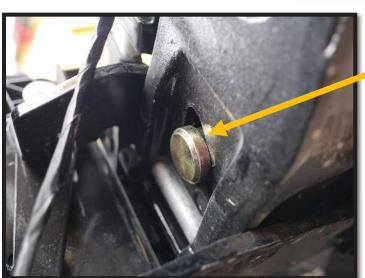
10. Insert the retaining clevis pin through the frame and bracket as shown. And insert the locking ring cotter pin to secure it.
