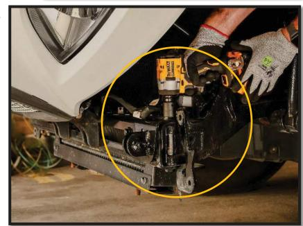
7. Put bumper back in place and torque these 2 bolts per side to factory spec
