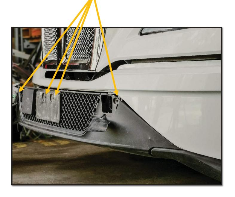
9. Install the Ex-Guard brackets through the bumper and into the receiver as shown.
