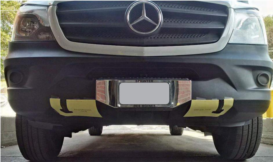
1) TAPE DRIVER AND PASSENGER SIDE BUMPER TEMPLATE INPLACE. START WITH THE EDGE OF PAPER AT THE CORNER AS SHOWN, AND INLINE WITH THE FORMED EDGE AS SHOWN.
