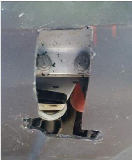
2) TAKE A JIG SAW OR KNIFE AND CUT OUT THE PROFILE ON BOTH SIDES.
