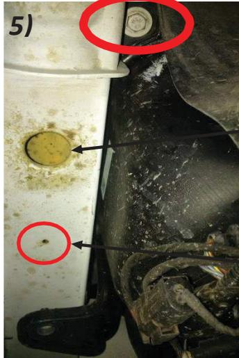
WHEN INSTALLING, USE THIS HOLE TO INSERT THE WRENCH SUPPLIED, WHICH WILL POSITION THE NUT OVER THE HOLE DRILLED IN-TO THE FRAME
