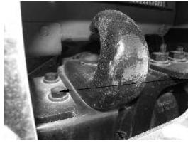
(1) LOCATE FRONT TOW HOOKS AND REMOVE, INSTALL BRACKETS AS SHOWN USING BOLTS SUPPLIED TORQUE TO 150 FT/LBS
