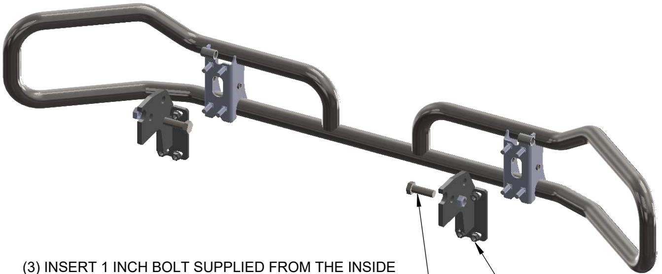
(3) INSERT 1 INCH BOLT SUPPLIED FROM THE INSIDE THROUGH THE BRACKET AND THROUGH THE HOLE IN THE FRAME WHERE THE CLEVIS USED TO BE. THREAD ON THE NUT TORQUE TO 680 FT LBS.
