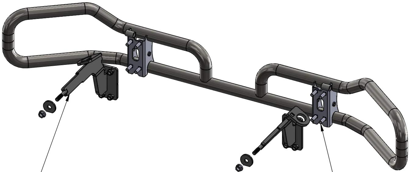
(1) INSERT THIS END INTO THE TOWHOOK RECEIVER, AS SEEN BELOW. PUT WASHER OVER BOLT, INSTALL NUT TORQUE TO 230 FT LBS.
