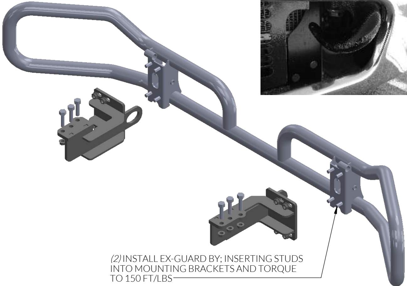
(2) INSTALL EX-GUARD BY; INSERTING STUDS INTO MOUNTING BRACKETS AND TORQUE TO 150 FT/LBS
