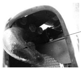
(1) REMOVE TOW HOOKS BY REMOVING 4 BOLTS PER SIDE AND INSTALLING BRACKETS AS SHOWN USING 3 BOLTS SUPPLIED. TORQUE TO 150 FT/LBS
