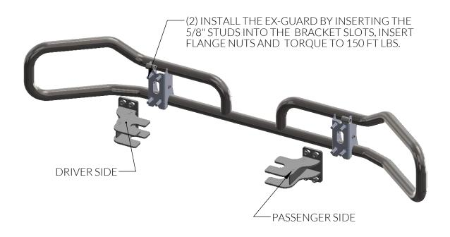
(2) ROTATE THE BRACKET INTO THE FRAME OF THE TRUCK.
